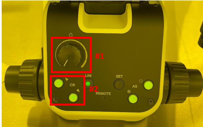
Figure 3. Light Intensity Knob (#1) and Objective Selection Buttons (#2)
