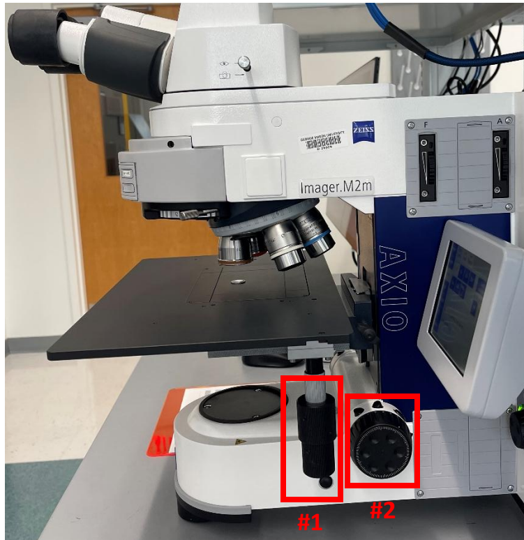
Figure 9. Microscope Showing Stage Controllers (#1) and Focus Adjustments (#2)
