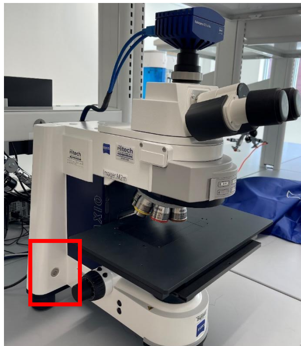
Figure 3. On/Off Button of the Microscope
